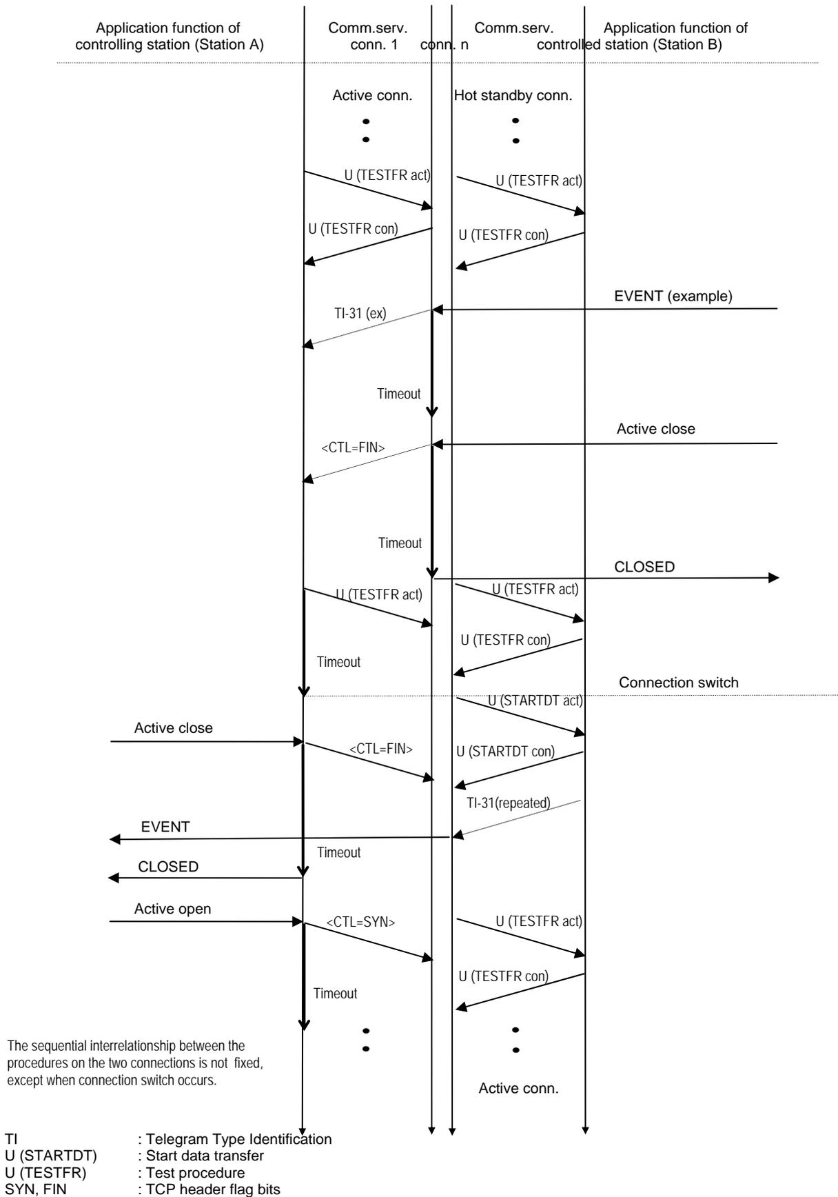
**Figure 7.6: Redundant connections - user data from controlled station**
