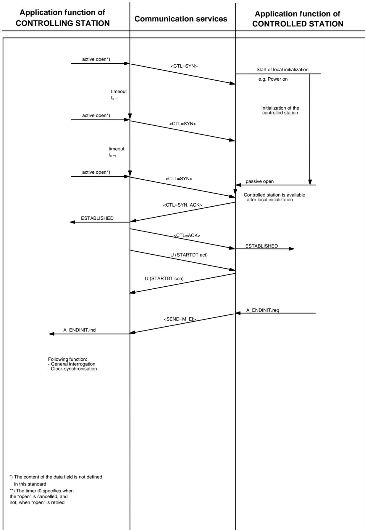
Figure 6.3: Local initialization of the controlled station
