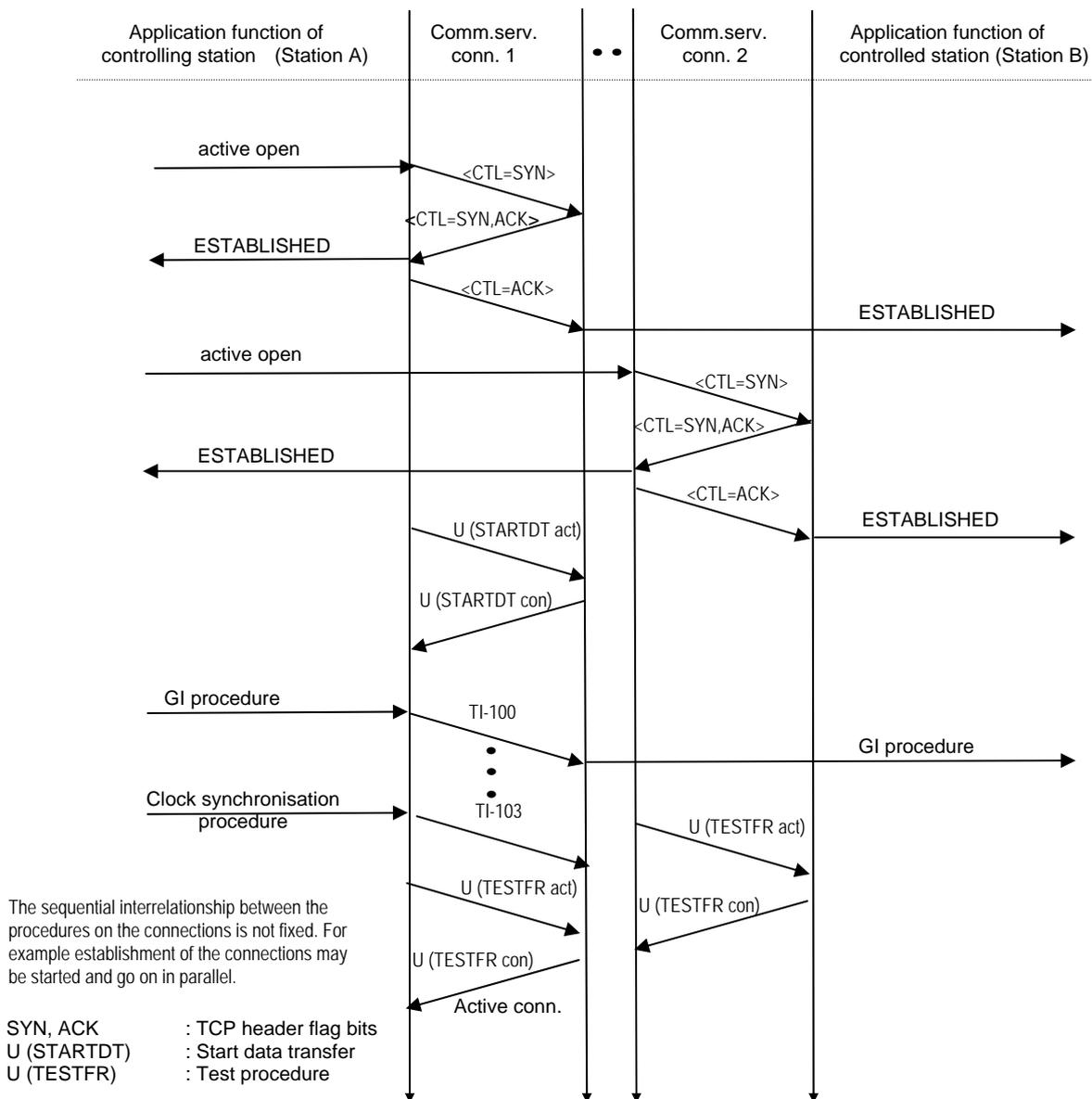
**Figure 7.3: Initialisation of controlling station with redundant connections**
