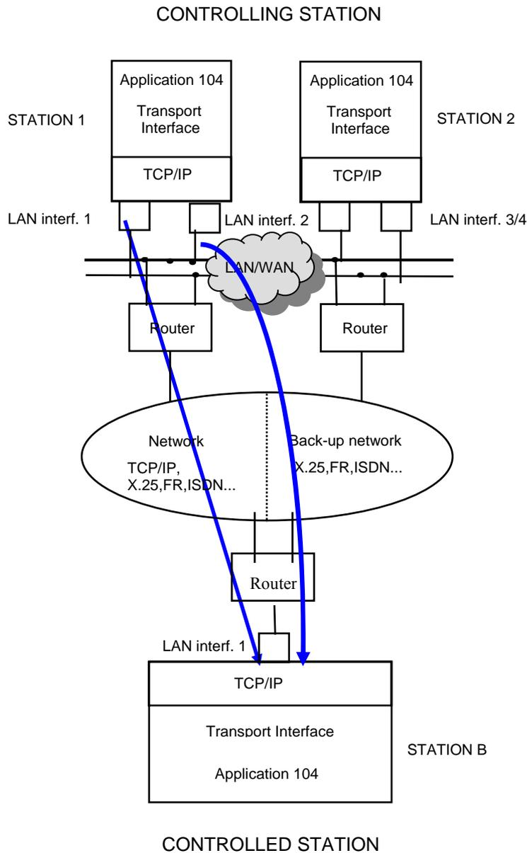
**Figure 7.1: Redundant system with a minimum of two possible connections from two interfaces at the front end**
